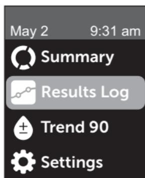
Up to four results are displayed on the screen, starting with the most recent.
