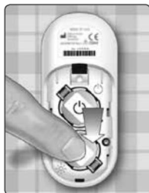
Replace the battery cover by sliding it upwards onto the meter.
