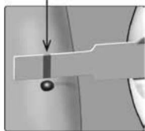
When it touches your sample, the test strip wicks blood into the channel.
