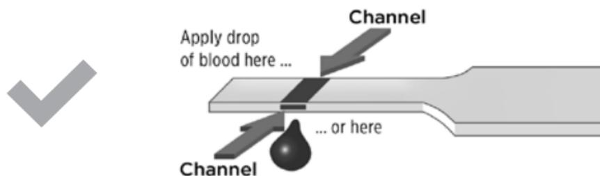
Blood should **not** be applied on the top of the test strip or to the end of the test strip.
