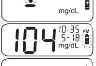
When the battery icon is flashing by itself on the display, **you cannot perform a test**. You must install a new battery before using your meter.
